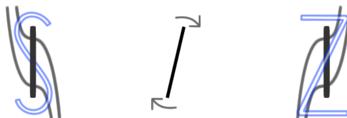
Figure 8: flipping a tablet to change it from S to Z (top view).
