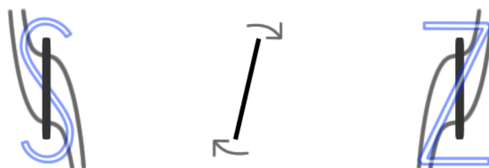
Figure 7: flipping a tablet to change it from S to Z (top view).
